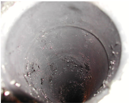
Fig. 4(b). Interior of the pipe (5 cm I.D.) after the second run at a higher oxygen concentration.
