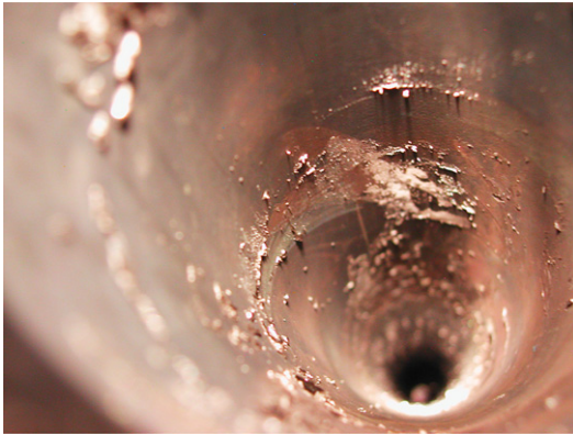
Fig. 4(a). Interior of the pipe (5 cm I.D.) after the first run at low oxygen concentration.
